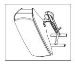
Gently pull the slack out of the wire and screw the shelf stand onto the back of the speaker in two places, as shown.
