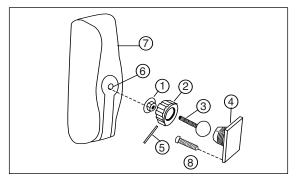
with the star washer side away from the ball. Refer to the exploded drawing for the proper orientation of these parts.
